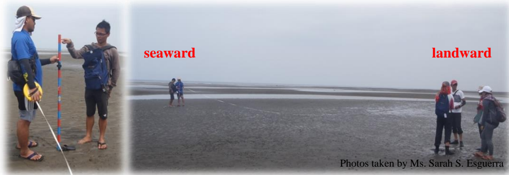
Figure 10. Reading made at seaward rod. Seaward reader points at the level (left) at which the landward reader sees the end of the landward rod align with the horizon. Value of the pointed level is recorded as a positive value.
