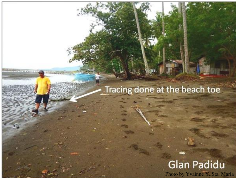
Figure 13. On coasts adjacent to fringing reefs or sandflat, shoreline tracing can be done at the beach toe, which is used as a shoreline change reference. On coasts adjacent to fringing reefs or sandflat, shoreline tracing can be done at the beach toe, which is used as a shoreline change reference. It is marked by a break in slope and drastic change in sediment size and composition.
