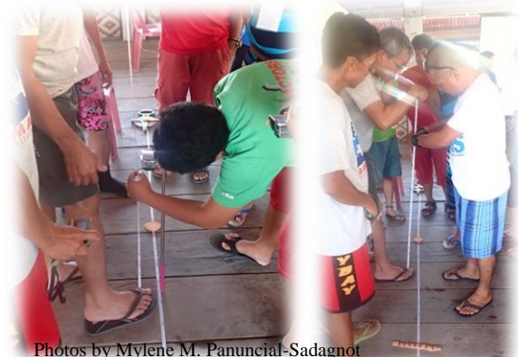
Figure 21. Camera calibration: Determining the height of monopod (left) and distance of camera (right) from surface to capture a 1x1m quadrat photo.
